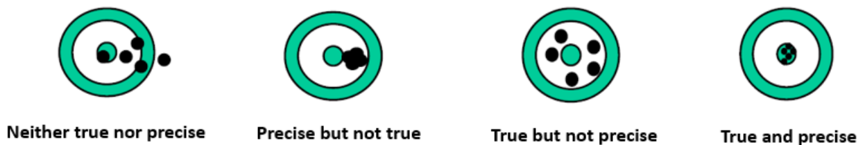
Figure 12 – Different types of uncertainty associated with laboratory measurements (modified from Ghestem and Lachenal, 2008).
